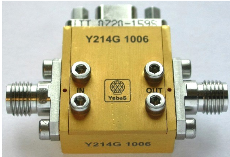
External view of the ultra-wide band cryogenic LNA developed.
