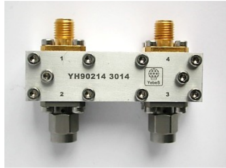
External view of one of the cryogenic 3 dB 90° hybrid couplers used in the balanced amplifiers together with the LNA on the left.
